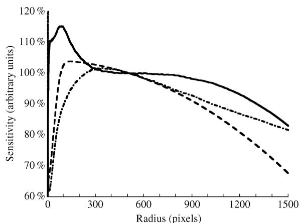
Fig. 3. Calibration tables for the DIP2030. The ratio (—) of the factory (---) default CorrectData table and the new (-·-) CorrectData tables is used by the software routine *RC.Scalepack.c* to correct previously scaled and merged data which were collected prior to installation of the new calibration table. The calibrations are scaled to 100% at  $r = 500$  pixels, which is approximately in the center of the flat region for the ratio of the two curves.
